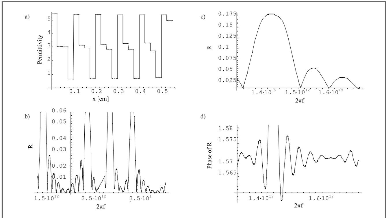
**Fig. 2.** Permittivity profile in the layer (a); reflection coefficient amplitude in dependence on the incident wave frequency (b), (c); reflection coefficient phase, equal to  $\pi$  at its maximum (d)
